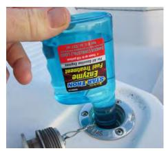
**SPIN:** "Tip #1: Ensure a tight seal, if water is found, dry the tank before refueling."
